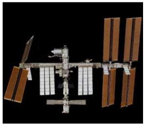
Over the course of the last 10 years of building the ISS, the look of it has changed dramatically growing from 2 modules to the size of 2 football field laid side by side by the time of its completion within the next 2 years. Pictures of the ISS at each stage of development can be found at <a href="http://spaceflight.nasa.gov/gallery/images/station/assembly/ndxpage1.html">http://spaceflight.nasa.gov/gallery/images/station/assembly/ndxpage1.html</a>.
